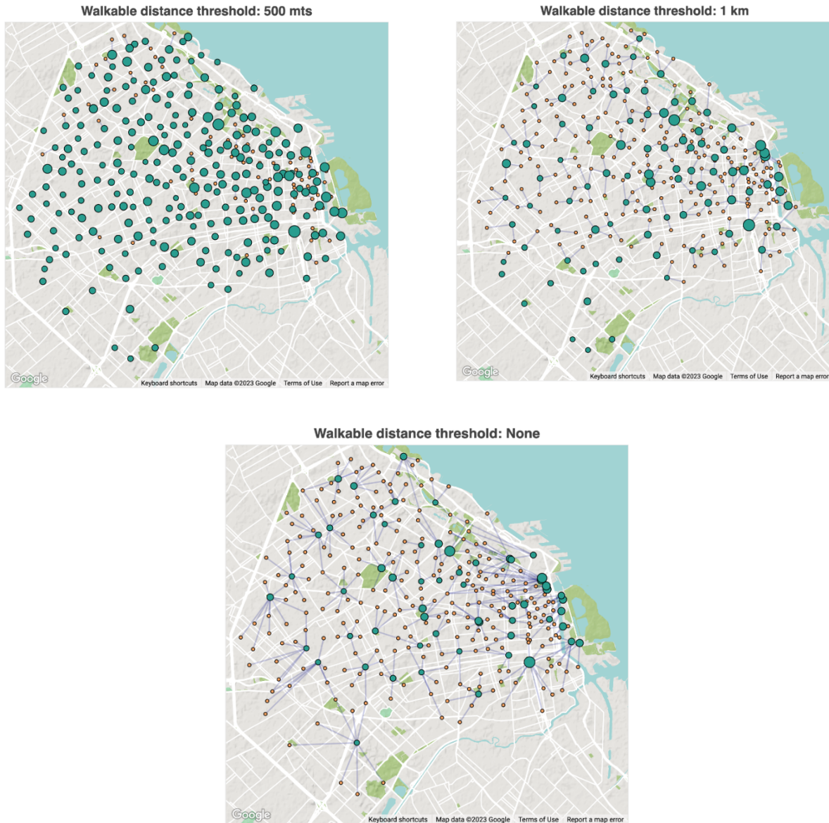
Figure 4.7: Graphical representation of different walkable distance thresholds: 500 mts (upper-left), 1 km (upper-right), none (bottom). Stations that appear to have no edges are in fact connected to the center of demand that is closest to them. Using CI upper bound demand prediction on weekdays.
