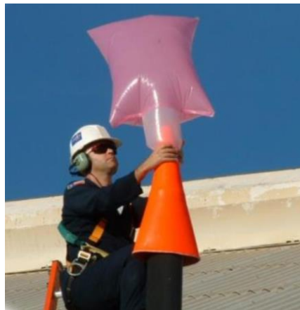
Figura 16 - Bolsa de volumen calibrado (Fuente: Climate and Clean Air Coalition & Oil and Gas Methane Partnership, 2017)
